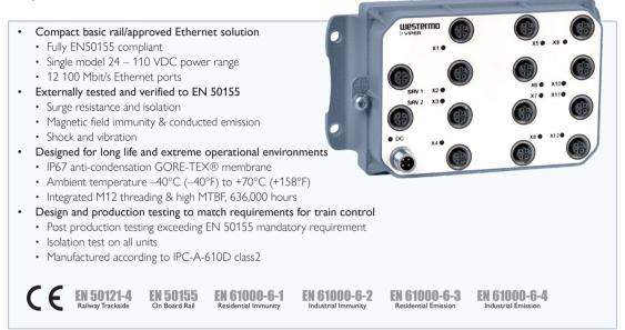
The Viper-012 is a basic unmanaged 12 port switch designed to meet the full requirements of the rail vehicle market. The incredibly compact and robust housing ensures the unit can be built into tight and environmentally hostile spaces.
