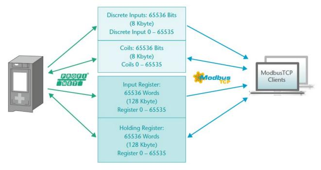
From the point of view of ModbusTCP communication, all coils, inputs and registers are always available in the PN/ModbusTCP coupler. So it is always possible to access all data types from address 0-65535.
