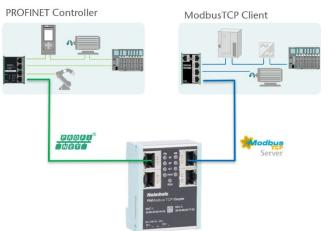
In addition to the PROFINET / ModbusTCP communication, the PN/ModbusTCP Coupler also makes an MQTT Publisher available on both network sides. In this way, the values exchanged via the gateway can also be distributed via MQTT to visualization or operating data recording systems.
